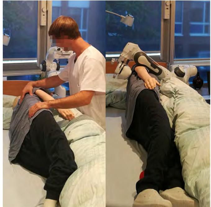
Fig. 1. Comparison between how a caregiver holds a patient and how our one-armed manipulator fulfills the same task. The nurse reaches from the front of the patient the shoulder and hip. It can also be seen here that not only the hand is used for the holding process.
