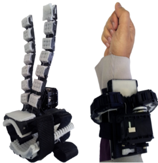
Fig. 3: The final prototype of double soft sixth finger, the device can be worn on the paretic arm through support base and elastic straps. It can be shaped into bracelet when being not used..
