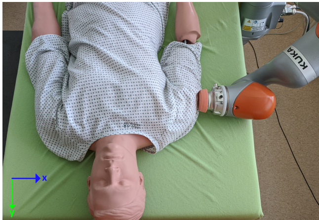
Fig. 5. The setup of the robotic load experiment where the robot tries to push the 80 kg weighing patient simulator without any external help. The pushing starts at about 2.4 seconds and ends after 12.2 seconds. The torque for every joint during the execution is measured.
