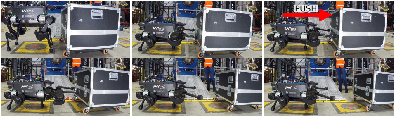
Fig. 7: The robot leaning on both prongs to push a box away. From top left: From a standing position (1), the robot lowers itself onto the prongs (2), which enables the front legs to be lifted from the ground. These front legs are used to push the box (3), which is pushed out of the way (4-6), clearing space for the robot to navigate onto the platform.
