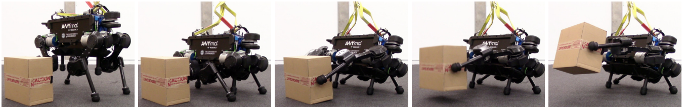
Fig. 9: Snapshots of box lifting experiment: support provided by the prongs frees up two of the legs for a manipulation task.
