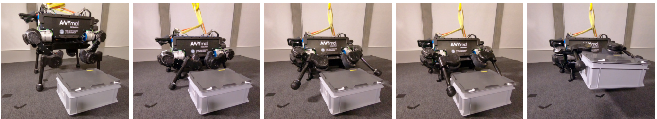
Fig. 10: Snapshots of a second box lifting experiment using a box with different dimensions.
