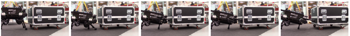
Fig. 8: The robot leaning on both prongs to push a box away. From top left: From a standing position (1), the robot lowers itself onto the prongs (2), which enables the front legs to be lifted from the ground. These front legs are used to push the box (3), which is pushed out of the way (4-5), creating a clear path.
