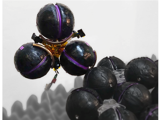
Fig. 1: FireAnt3D climbs atop a collection of its peers by flipping about strong connections it made using its 3D continuous docks. The robot attaches to like robots without alignment, allowing for simple locomotion.
