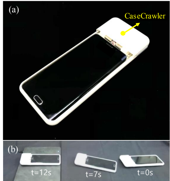
Fig. 1. (a) The CaseCrawler employed as a movable platform. (b) A smartphone with a movable platform moving toward a wireless charging plate by itself.
