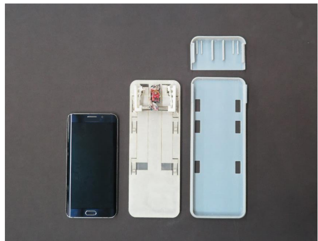
Fig. 10. PhoneCaseBot, which consists of a CaseCrawler, a protective shell, and electronics. Mobility is given to the smartphone by attaching a portable crawler with high payload capacity. As a result, the smartphone can crawl to reach the wireless charger.
