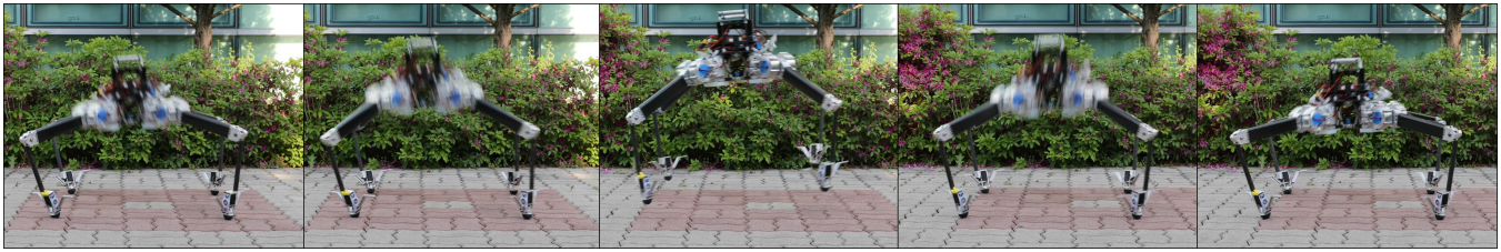
Fig. 9: A time series depicting one full pronking gait cycle. The robot is moving at 0.3 m/s to the left.
