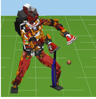
Fig. 11. Dynamics simulation environment The simulator handles the robot dynamics simulation and the camera images simulation. As a ball is thrown from 4[m] from the robot, the robot performs a motion using our proposed real-time system.
