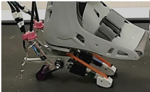
Figure 1. Mechanism of the Ankle-foot prosthesis end-effector: (Top) CAD model with detailed description, and (Bottom) Hardware implementation. We printed strain relief assembly, toes (white part), etc. We improved the robustness of the heel (purple part) using carbon fiber. Pulling the inner cable provided plantarflexion, releasing the inner cable and using rubber bands between screws on toes and the main part was for dorsiflexion.
