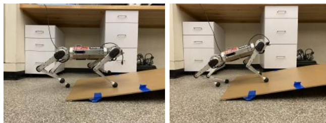
Fig. 10. Posture pitch adjustment due to sloped terrain. Mini-Cheetah Vision walking onto a sloped surface: (a) without pitch posture adjustment, and (b) with pitch posture adjustment added to the desired pitch of the body.
