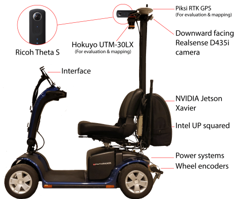
Fig. 4: Hardware overview of retrofitted mobility scooter
