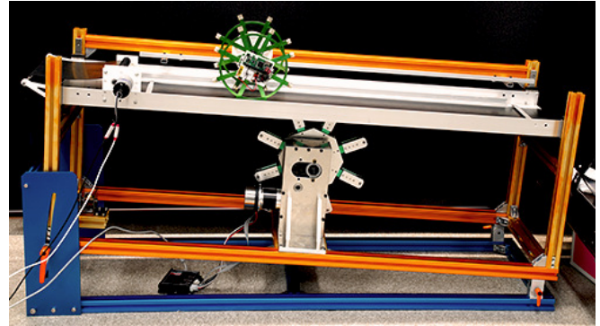
Fig. 1: Prototype experimental system of vibratory conveyor system
