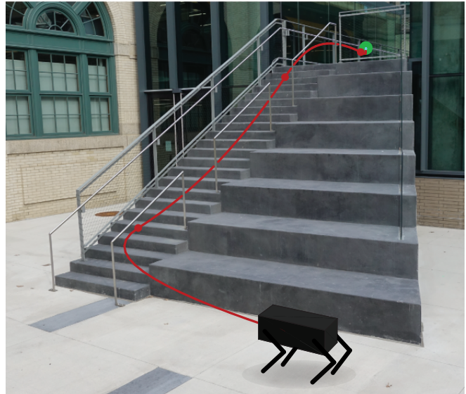
Fig. 1. Demonstration of the presented algorithm generating a long dynamical plan over terrain challenging for a legged robot in under three seconds. The trajectory from the start pose to the goal (green circle) is overlaid on an image of the environment used to generate the plan.
