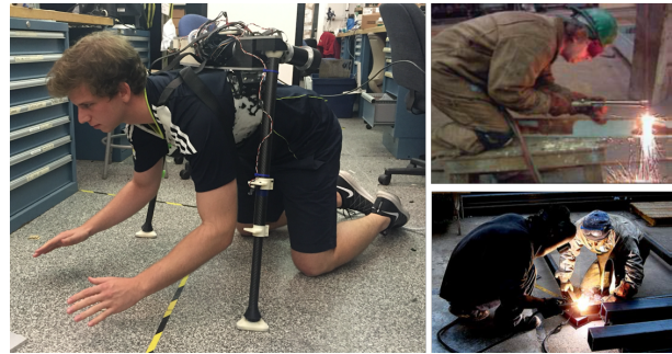
Fig. 1. SuperLimb supporting a human working on the floor (left) [12] and welders in ergonomically poor postures while working (right) [13]
