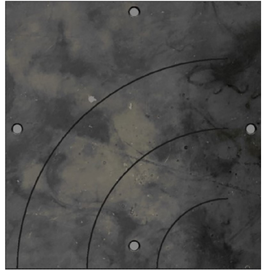
Fig. 2. Steel heat treatment mold for Nitinol wires with three different radii. The Nitinol wires are put in the grooves and then put in the oven at 500° C for about 30 minutes and then quenched to get the constant pre-curvatures.
