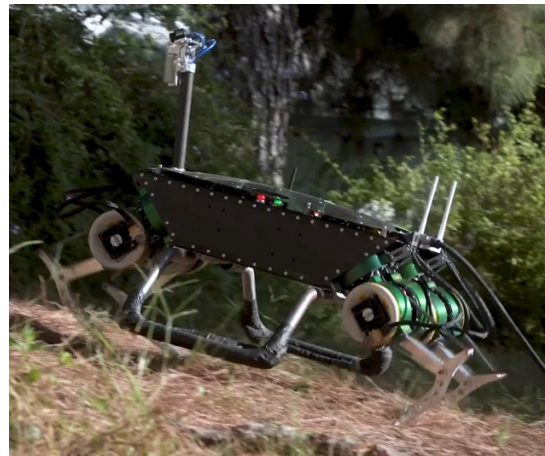
Fig. 12: LLAMA able to (a) walk over various debris without any vision and can recover from disturbances and (b) walk and strafe up and down inclines of up to 15 degrees
