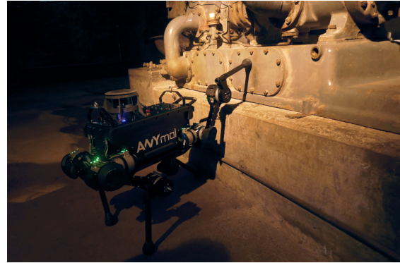
Fig. 1. ANYmal using its foot to measure the vibrations of a piece of mining equipment. Tasks such as this might require localization even when vision cannot be used. By exploiting prior knowledge of the 3D environment, the robot could use contact events to localize itself. Source: ETH Zurich.
