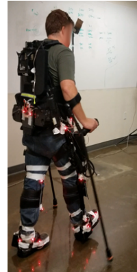
Fig. 1. Ekso GT exoskeleton. This work considers state estimation and gait phase detection for lower-extremity exoskeletons and tests the framework on data from human-subject tests with the Ekso GT.
