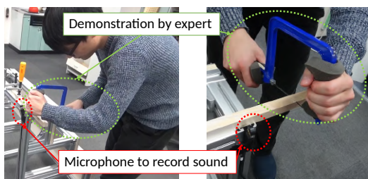
Fig. 5: The expert operates the hacksaw and samples the sound to train the NN to determine whether the operation sound of the hacksaw is close to the sound of expert's operation.
