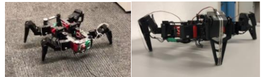
Figure 12. MW snapshots with (right) and without (left) pressure sensors.
