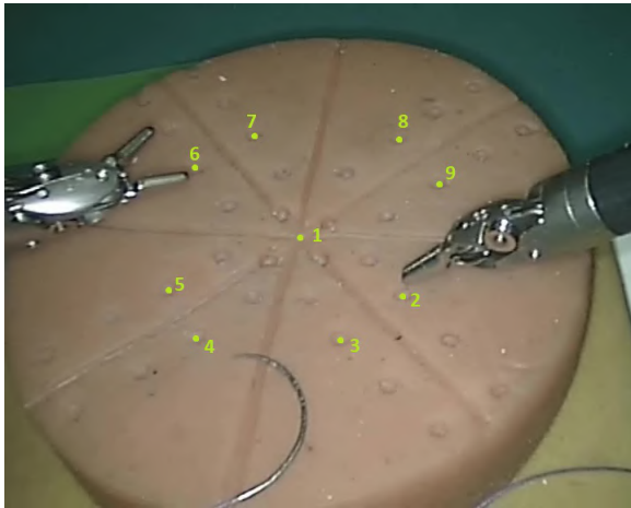
Fig. 3: Right camera endoscope image extracted from trial 22 showing the rotated position of the phantom. Numbered points indicate ordered fiducials used for spatial calibration.
