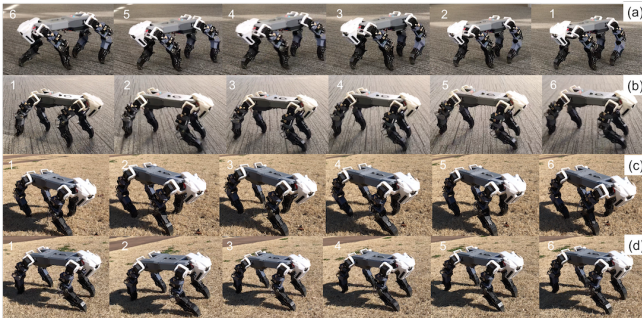
Fig. 10. Snapshots of the robots performance shows the dynamic gait pattern during leg injury: a) the robots performance on the flat terrain with a forelimb injury; b) the robots performance on flat terrain with a hindlimb injury; c) the robots performance on natural terrain with a forelimb injury; d) the robots performance on natural terrain with a hindlimb injury.
