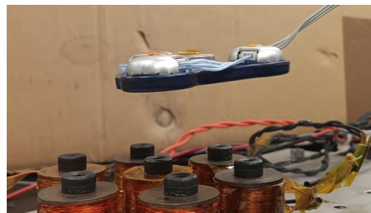
Fig. 4. Levitated magnet with iron core coils
