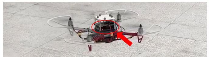
Fig. 2. Hovering test of low-level flight control. The red circle indicates the location of the FPGA-based FCU.
