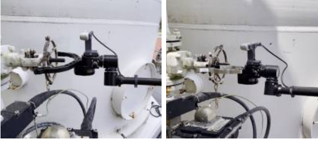
(a) Approach 1: Grab from outside (b) Approach 2: Grip on the ring
