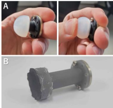
Figure 17. Optimization of the axis arm end to enhance friction [15].
