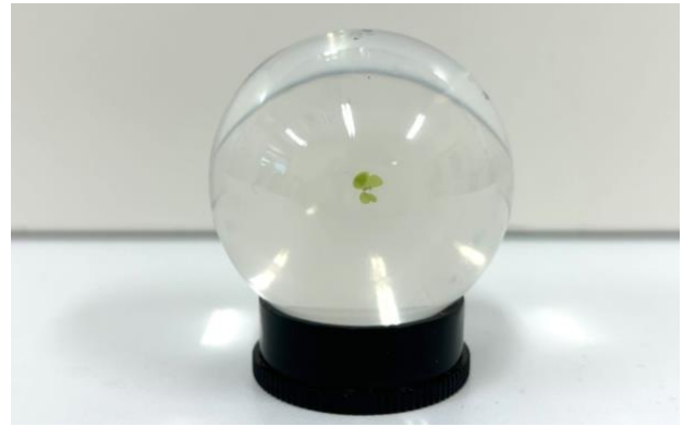
Figure 20. 3 {mm} clover leaf placed in a transparent gel at the middle of a plastic sphere of diameter 40 {mm} [15].
