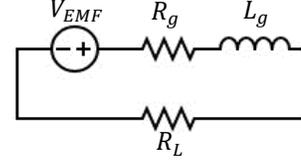
Fig. 2 Schematic of the knee energy harvester
