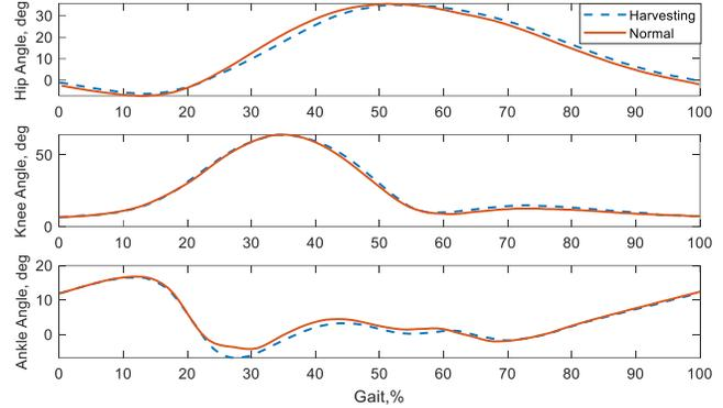
Fig. 8 Lower limb kinematics while walking at 4 km/h with and without the harvesting system
