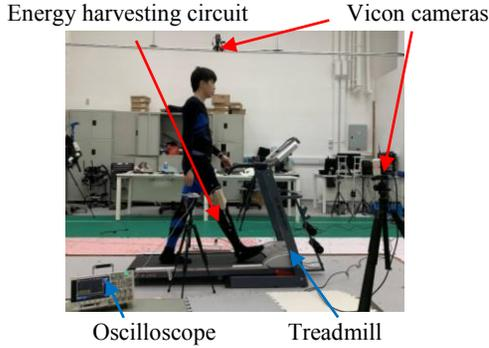
Fig. 6 Experimental setup for harvester evaluation
