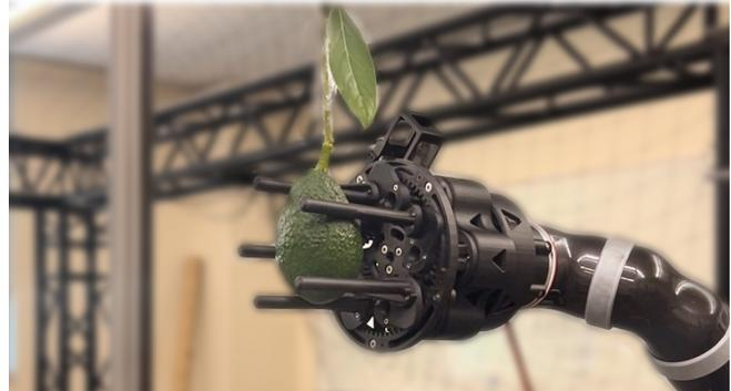
Fig. 1. We developed a custom-built end-effector attached to an off-the-shelf 6-DOF robotic arm for avocado harvesting.
