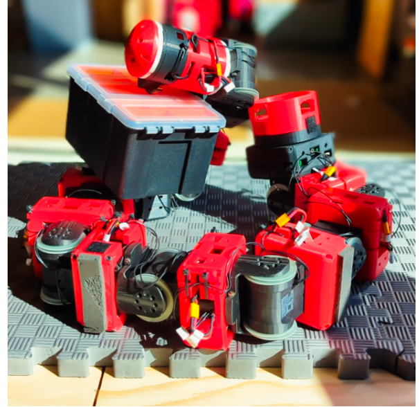
Fig. 1. Illustrates loco-manipulation problem concerning carrying a box with COBRA
