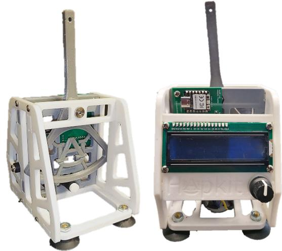
Fig. 1. This paper presents an innovative design for the Auburn Haptic Paddle, which supports increased accessibility via 3D-printed and commercial-off-the-shelf components (CoTS) to facilitate the integration of data-driven control in system-dynamics education.
