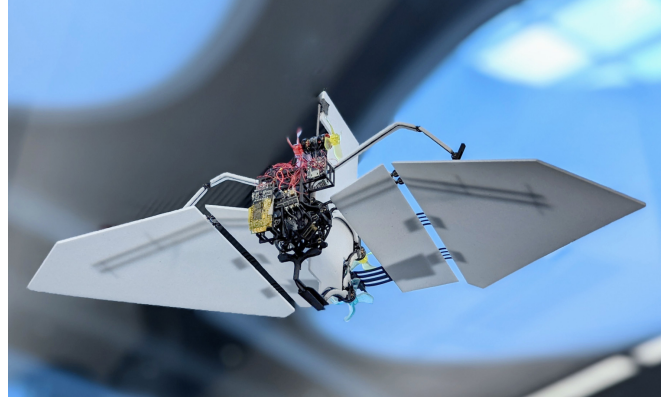
Fig. 1. Aerobat, a small flapping-wing, bioinspired bat robot with morphing wings.
