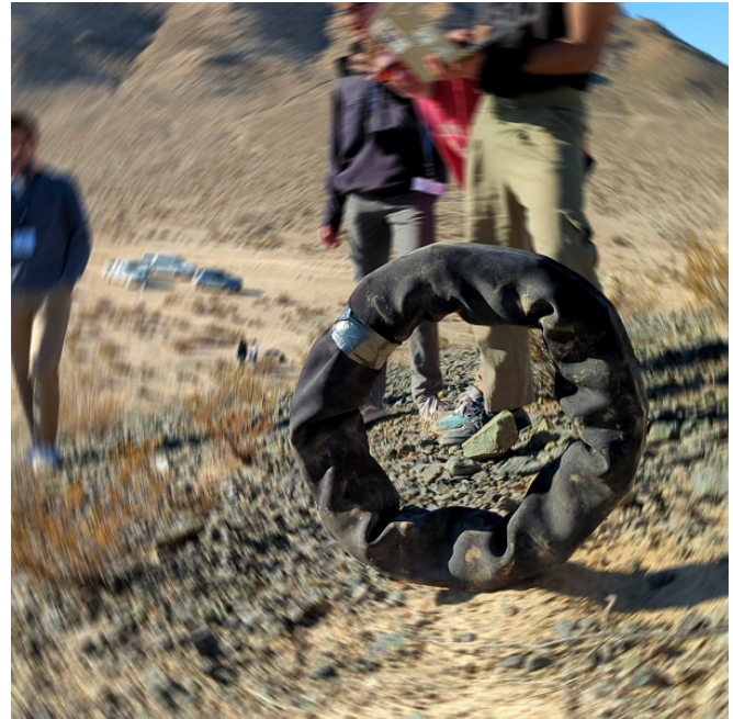
Fig. 1. Shows COBRA, Crater Observing Bio-inspired Rolling Articulator, performing tumbling locomotion in NASA's Innovative Advanced Concept Competitions in Pasadena, California, in November 2022.
