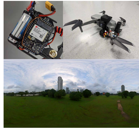
Fig. 2. Top Left: RTK GPS logger used for ground truth collection. Top Right: Drone with mounted Insta360 Sphere camera and RTK GPS logger. Bottom: Example of collected panoramic 360 image in 2:1 equirectangular format (from Kallang Riverside).
