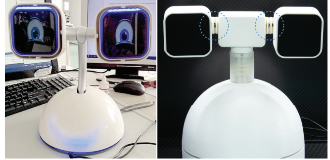
Fig. 1. (left) HARU as first presented in [3] and (right) the revised prototype structure incorporating soft joints in the head and eye structures, for enabling life-like motions and enhancing safety during interactions. This work is focused on the development and modeling of a soft continuum actuator for enabling the yaw motion of the eye structures (highlighted in blue and conceptually presented in Fig. 2).
