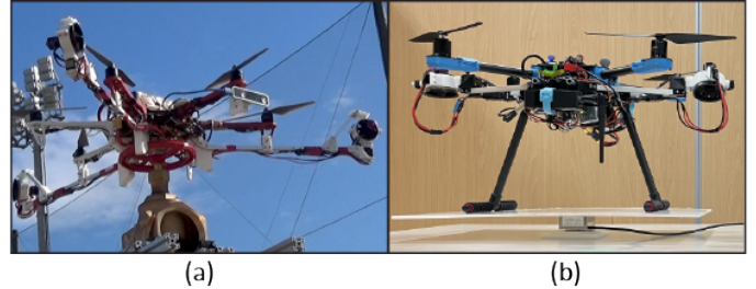
Fig. 1. Add-on thrust vectoring device configurations: (a) High torque configuration. (b) Dual torque configuration
