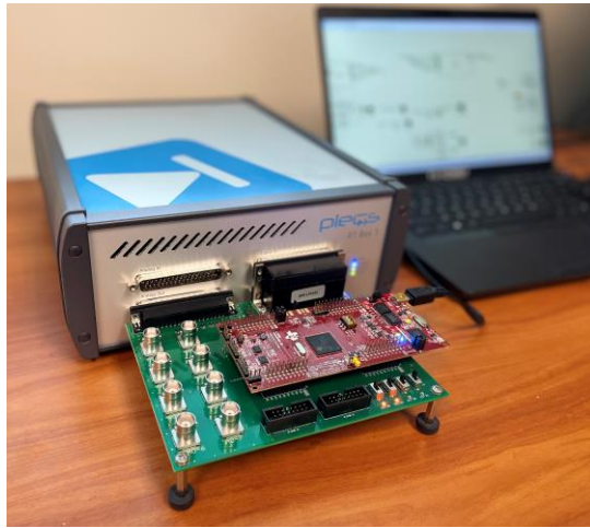
Figure 6. Hardware-in-the-Loop setup consists of a Plexim RT Box, a TI TMS320F28379D Evaluation Board, a LaunchPad Interface, and a PC for code generation.
