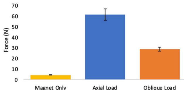
Figure 5. Experimental testing of MagLink's maximum strength under axial and oblique loads (top). The result comparison of magnet strength with and without engagement of the MagLink (mean and standard variation) of nine tests.
