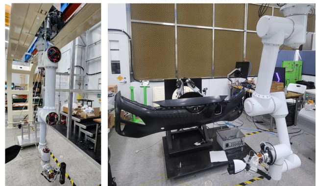
Fig. 3. Prototype of the EV charging robot system
