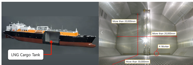
Fig. 1. The left figure shows a general LNG ship. The right figure shows a cargo tank. Generally, a ship has 4-6 tanks.
