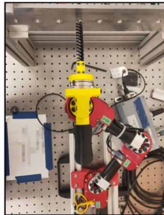
Fig.1, Schematic drawing (left) and top view (right) of the experimental SEA robot. The cleaning task for a specific pilot hole consists of letting the brush achieve a periodic forward-and-backward motion with stroke length d , which should be perpendicular to the plate, i.e., the end-effector orientation \theta = \pi/2 rad. The controlled outputs are the local joint angles \theta_1, \theta_2, \theta_3 .
