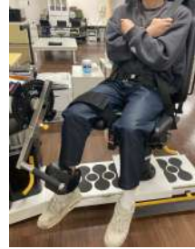
Fig. 9: Measurement of knee joint torque in Cybex
