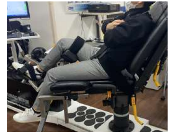
Fig. 10: Measurement of ankle joint torque in Cybex
