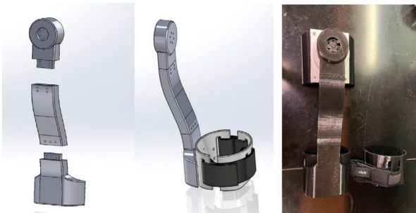
Fig. 3. Left: the exploded view of the hip component model. Center and Right: design assembly and 3D print of the hip component and thigh brace
