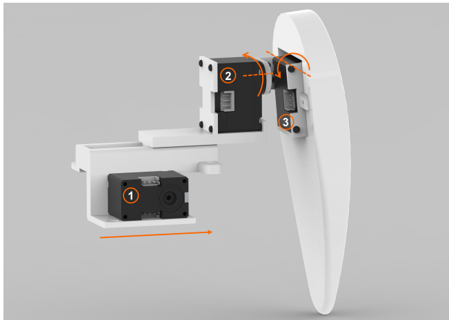
Fig. 6. An overview of the 3 DoF arm mechanism, with highlighted motors and resulting motions.
