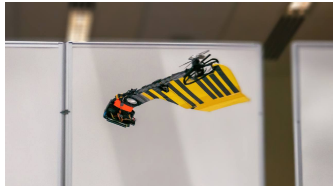
Fig. 1: Image of the SICARO flying in the clockwise direction, the front motor stopped to prevent counter rotation
