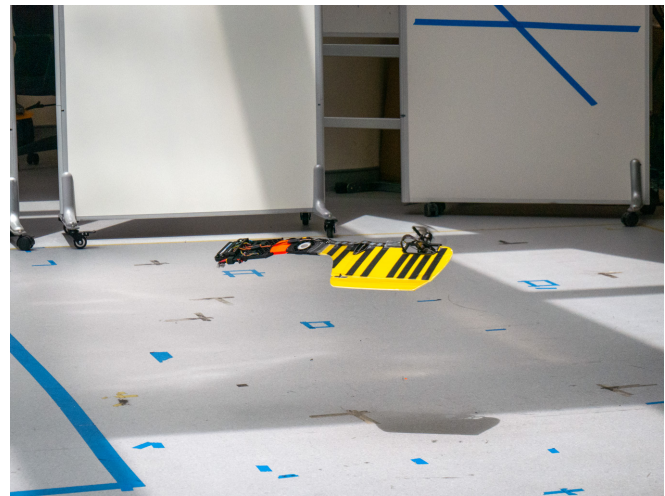
Fig. 23: Counter-clockwise rotating flight using the front motor in experiment
