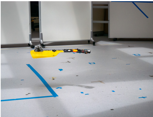
Fig. 22: Clockwise rotating flight using the back motor in experiment
