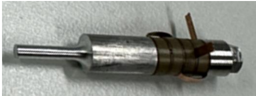
Fig. 7 The fabricated prototype of the miniature ultrasonic transducer
