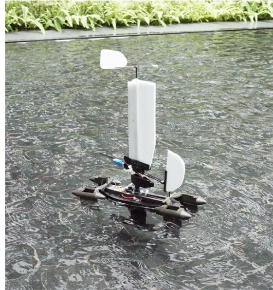
Fig. 1. Proposed novel design of micro-scale sailboat, featuring a bi-directional hull and a freely-rotating rigid wing sail.
