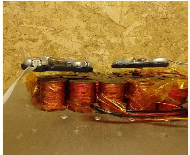
Fig. 5. Two magnets levitated independently with parallel orientation by single coil array
