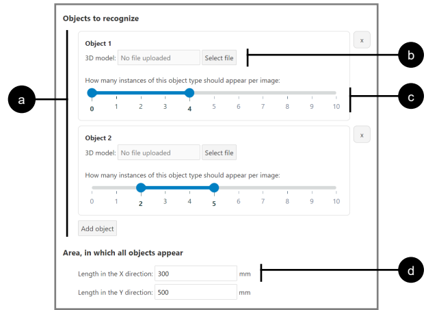
Fig. 4. Example form with form components highlighted: a) DynamicList , b) 3DModelInput , c) RangeInput , d) NumberInput . The DynamicList component allows End Users to create an arbitrarily long list of objects, e.g., so that they can specify objects to be recognized in a task without the Data Scientist having to specify how many objects there will be beforehand. For each object, all form components nested within the DynamicList component are loaded so that the End User can set attributes for each object.
