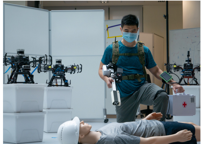
Fig. 1: A robotic system of systems that features a rescuer (the human operator) and three aerial robots that would enable better situational awareness and prompt access to casualty (mannequin) in a USAR scenario.
