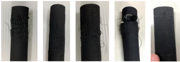
Fig. 8 Broken condition of the actuators. When p = 2.9, 2.4, 1.2, and 0.8 mm, yarn breakage occurred, and the rubber expanded at the point where it was no yarn constrained, and after deflating, the yarn was exposed from the rubber. At p = 0.4 mm, a small hole appeared in the rubber.
